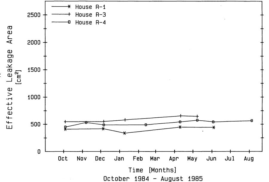
Fig. 2: Effective Leakage Area vs. Time for Reno Houses
