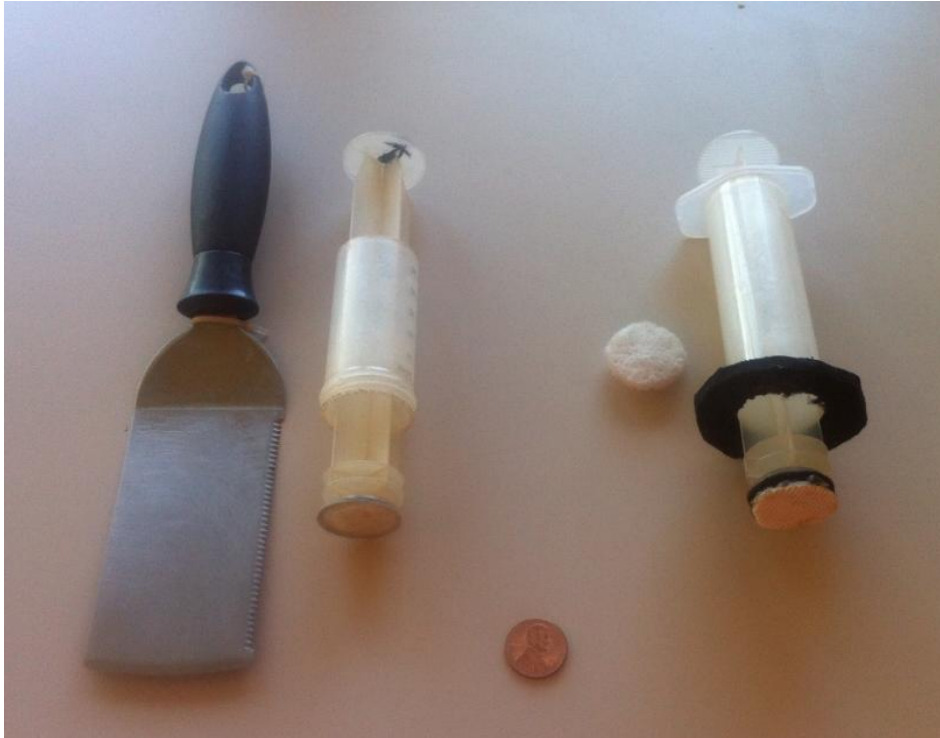
Figure 8: Benthic algae sampling tools. The sampler and spatula used to collect soft substrate algae samples is on the left. An example of the sampler used to collect algae samples from cobbles and boulders is on the right, along with an example of an abrasive scrubbing disc. The penny (diameter of 1.9 cm) is included for scale.
