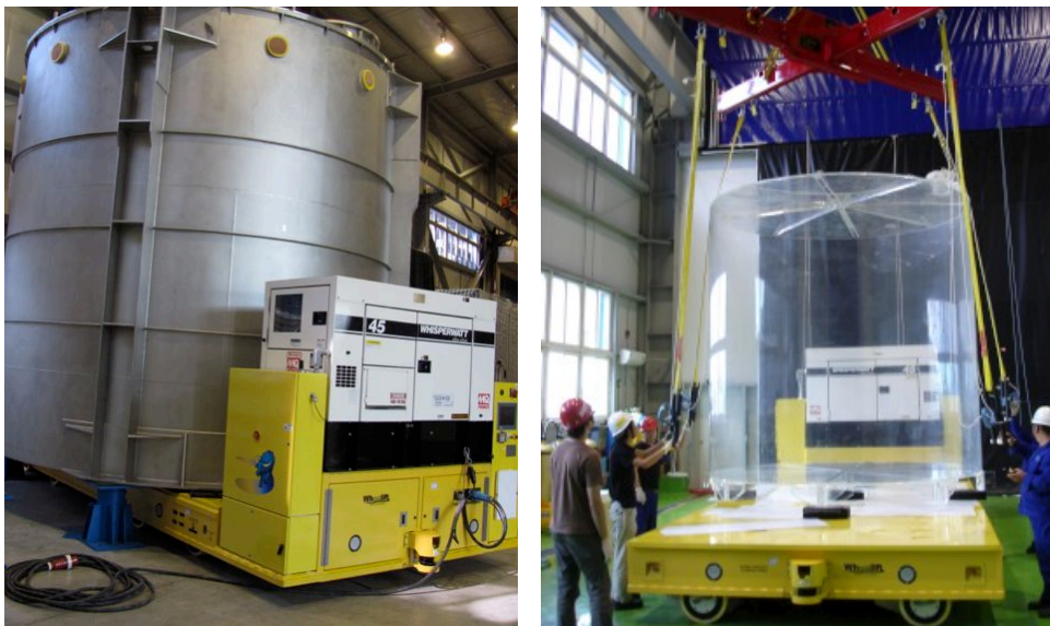
Figure 7. (left) The SSV is being lifted by the AGV from storage stands prior to transport to the cleaning room. (right) An IAV has been lifted onto the AGV after cleaning.
