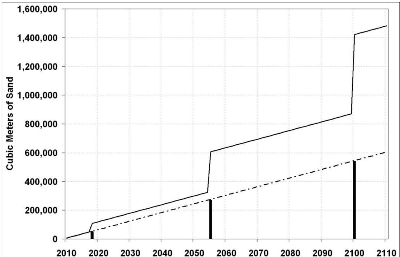
Figure 3. Sand volumes per kilometer of beach needed to keep pace with hypothetical sea-level rise over the next century (starting in 2010) of 50 cm/cy. Straight broken line: Cumulative amount of “regular nourishment” assuming 6,000 m<sup>3</sup>/yr; Solid bars: Three additional wave-storm replenishments in years 8, 45, and 90 (see text); Solid line: Total cumulative amount.
