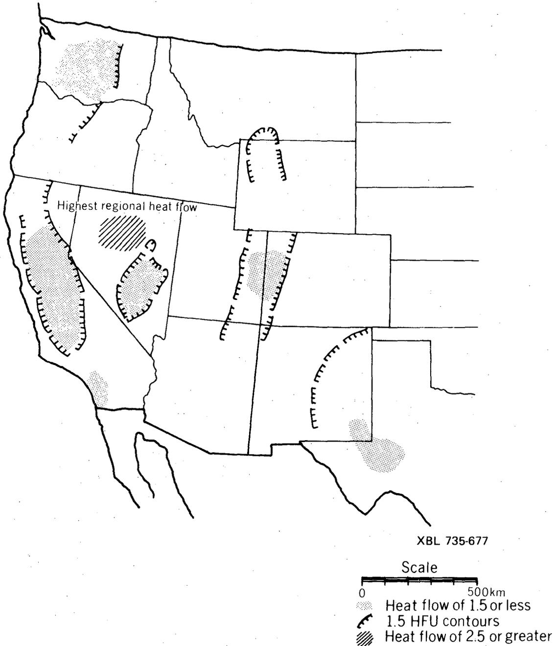
Figure 1 Regional heat flow in the western U.S. (after Sass et al., 1971). The stippled areas have heat flows estimated less than  $1.5 \mu\text{cal cm}^{-1}$ , (hfu) while in the dashed area, the "Battle Mountain High" heat flow probably exceeds 2.5 hfu. Hachured lines indicate the fairly well defined position of the 1.5 hfu contour.
