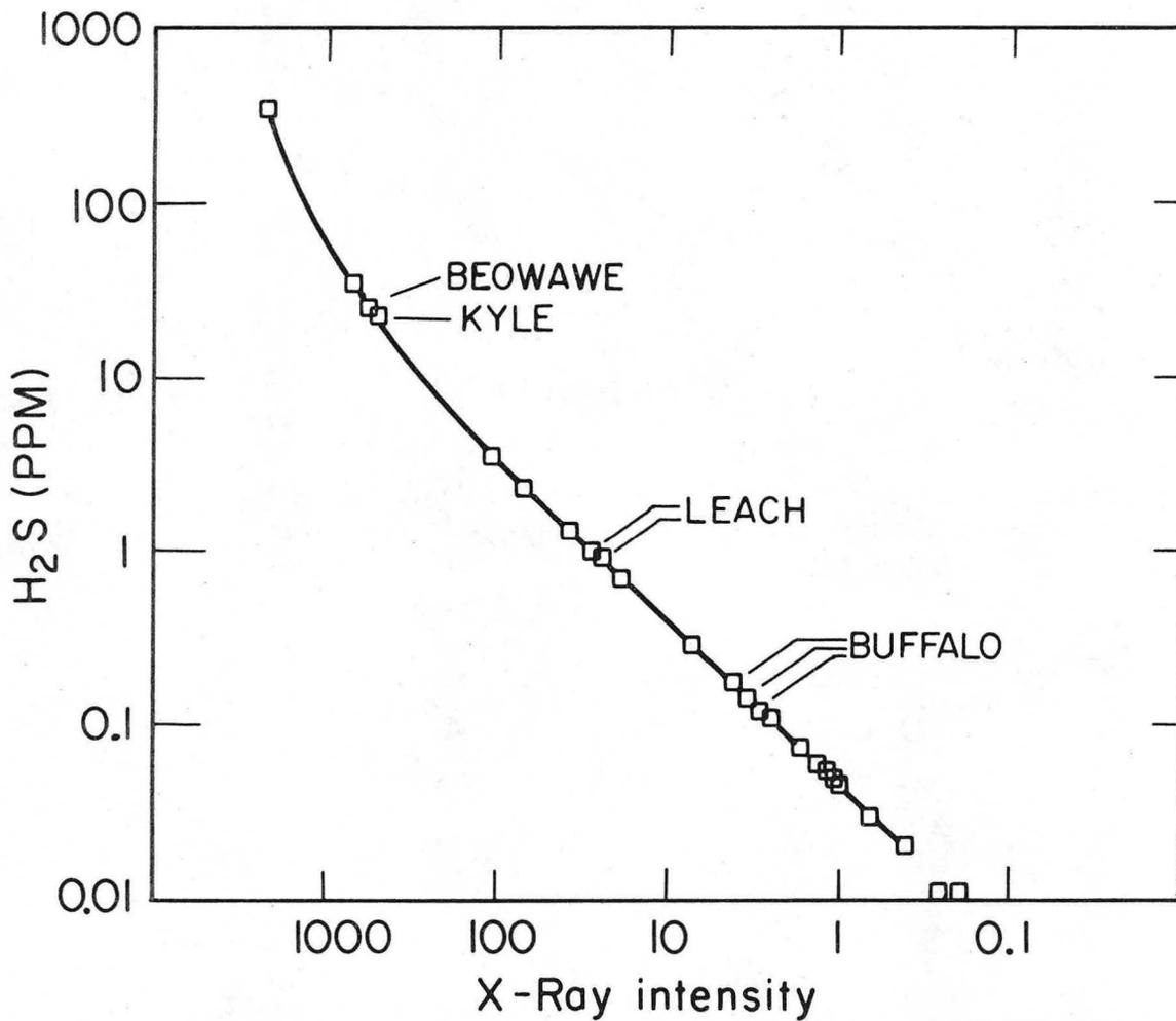
Figure 11 Calibration curve for equivalent H<sub>2</sub>S contents of spring waters, using the non-dispersive x-ray fluorescence method.
