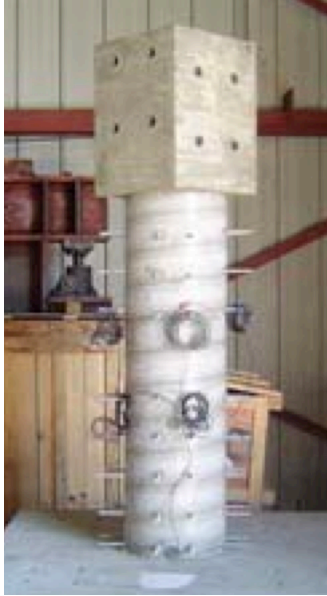
Figure 3-11: Threaded rods for measuring column curvature
