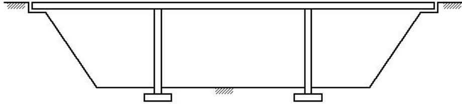
Figure 1-1: Generalized Bridge with Spread Footings
