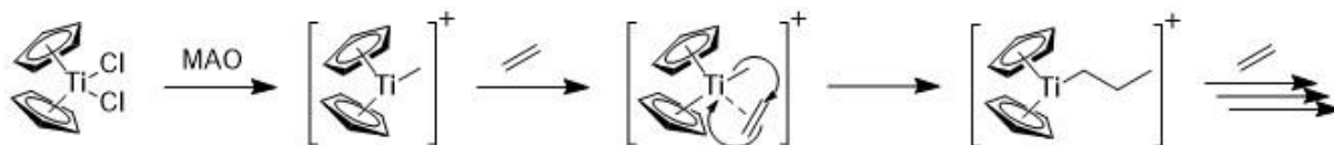
Scheme 1.1 Mechanism of ethylene polymerization by \text{Cp}_2\text{TiCl}_2 and MAO cocatalyst to afford HDPE 8
