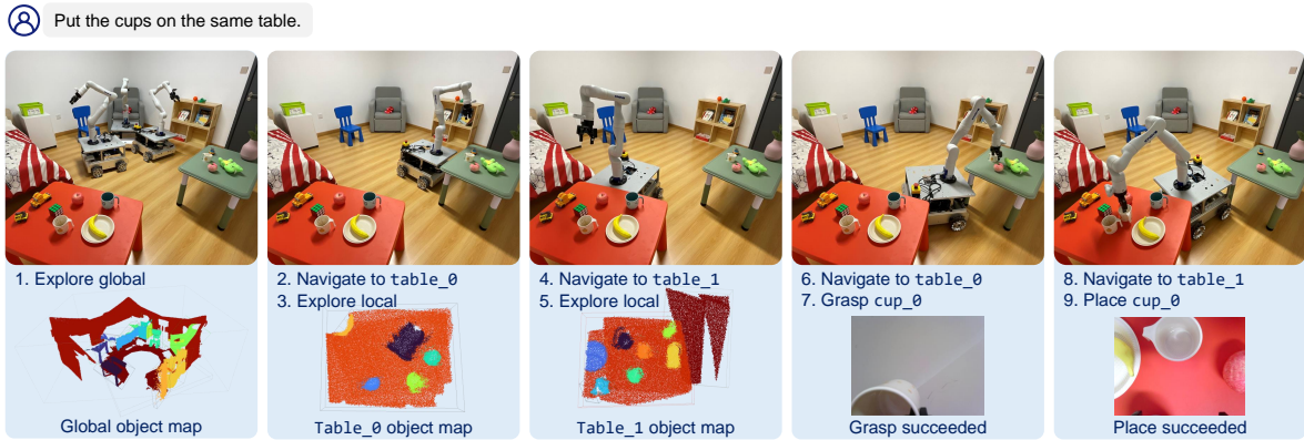
Figure 3.4: A step-by-step visualization of COME-robot’s task execution in GATHER CUPS.
