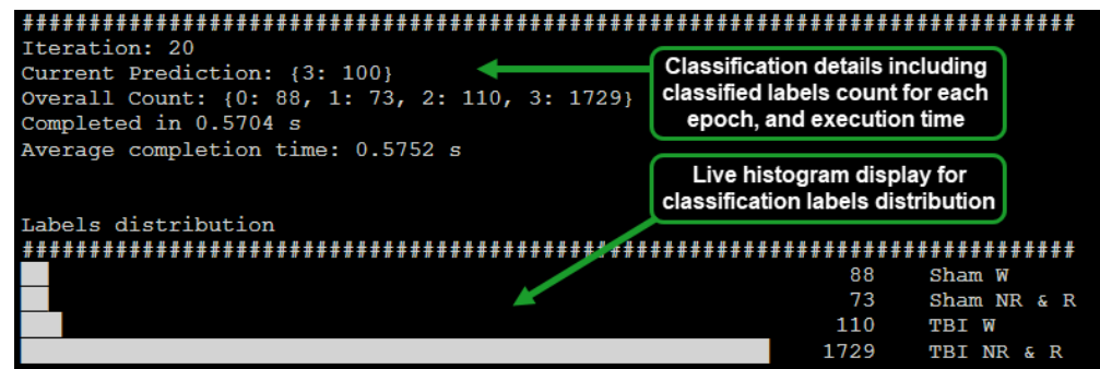
Figure 3. Live classification display for the RPi based system (64 s epoch, batch size: 100).
