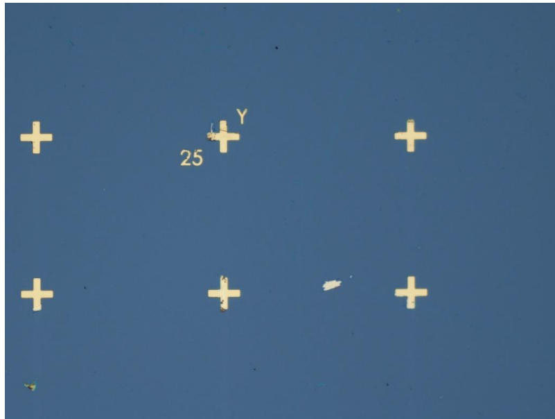
Figure 3.5: Optical image of SiO 2 /Si wafer with pre-patterned marker.
