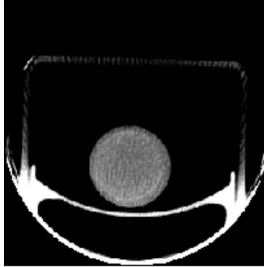
Figure 5.5: Example transaxial image of sphere scanned within the microCT scanner. The size of this slice is 256 x 256 (0.2 mm x 0.2 mm). The centroid of this sphere is the quantity of interest, but the nonzero voxels of the bed and nonuniformity within the sphere precludes this. Additional image processing must be performed before the geometrical centroid can be calculated.
