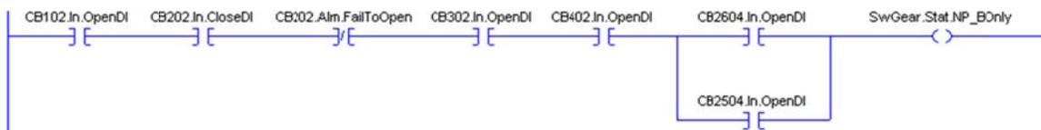
The test that found the bug is designed to test one of the system failure scenarios. The initial system state of this scenario is NP-BFeedA, the first trigger event is the utility power B failure, the second trigger event in this test is the CB202 "failed to open" alarm,
