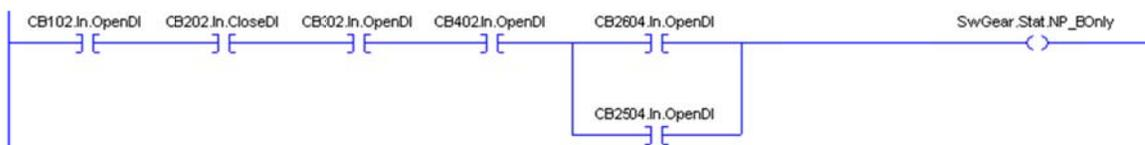
In order to determine if the switchgear is in the NP\_BOnly state, checking the circuit breakers' states is necessary but not sufficient. You also need to check CB202's failure condition in this case. If CB202 "failed to open" alarm is active then the switchgear should be in the Plant Dark state instead of in the NP\_BOnly state. The correct version of the ladder code is as follows:
