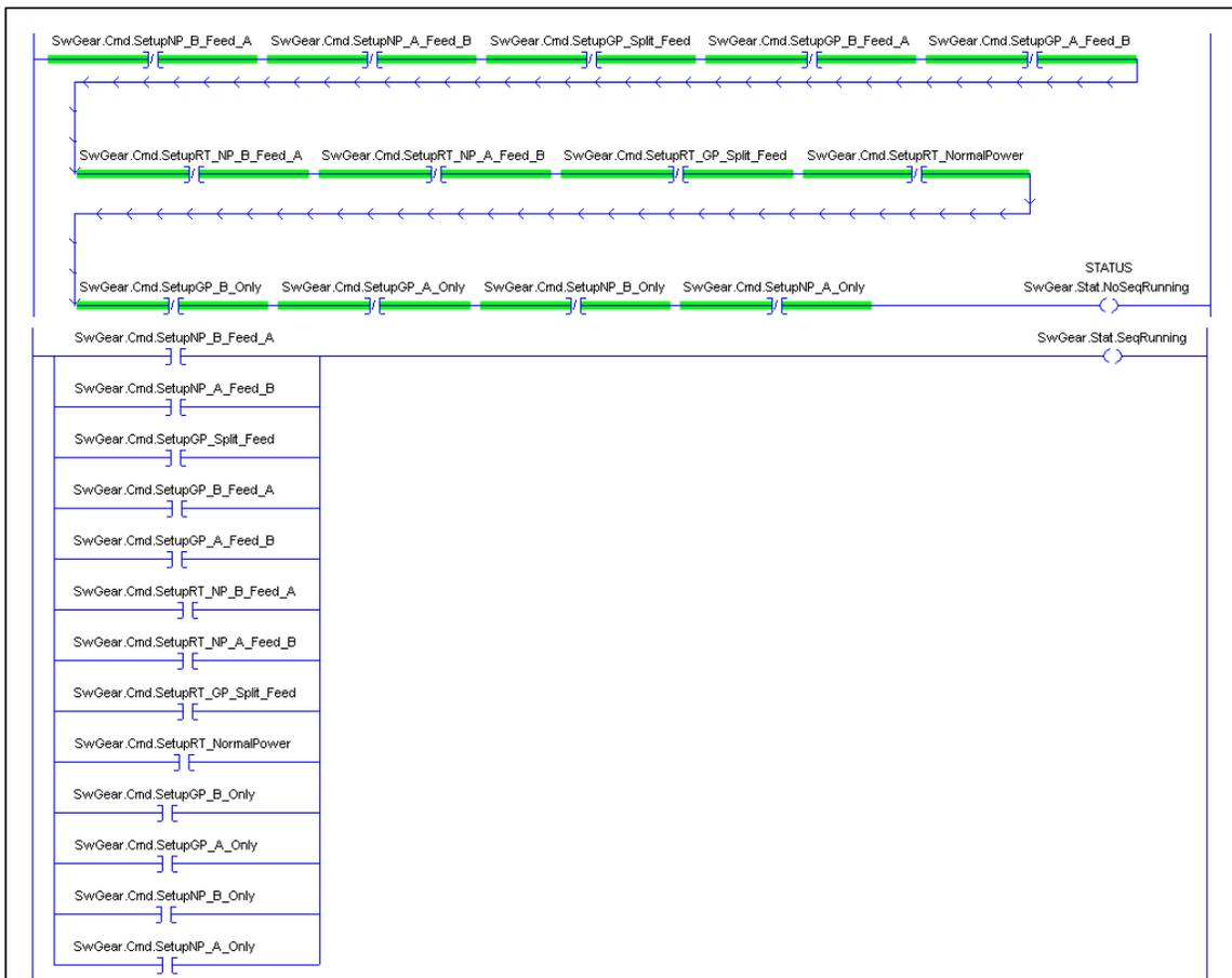
**Figure 5.13: Fixes for the ladder code in Figure 5.12.**
