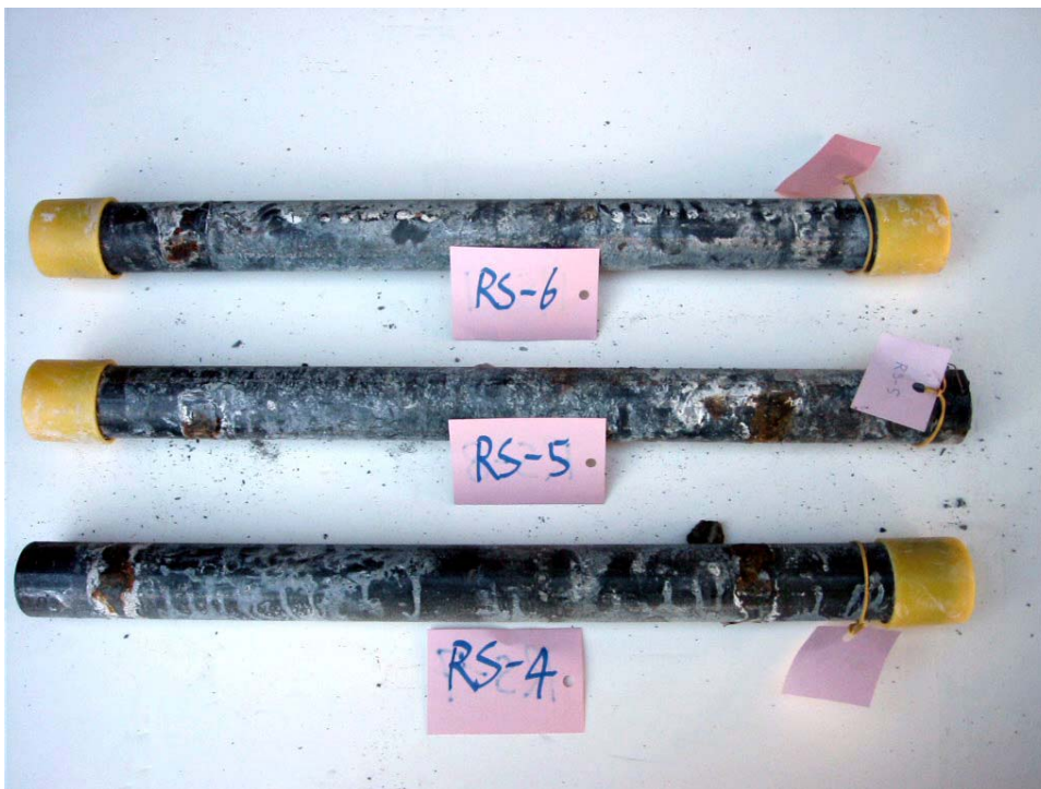
Figure 22. Corrosion along the carbon steel bars.
