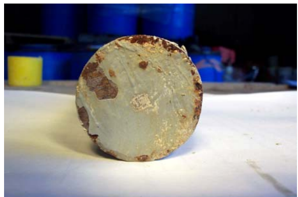
Figure 41. Epoxy-coated dowel (gray). (a) General view of the center region; (b) Corroded edges at the end of dowels.
