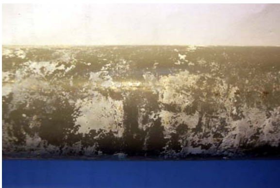
Figure 41. Epoxy-coated dowel (gray). (a) General view of the center region; (b) Corroded edges at the end of dowels.
