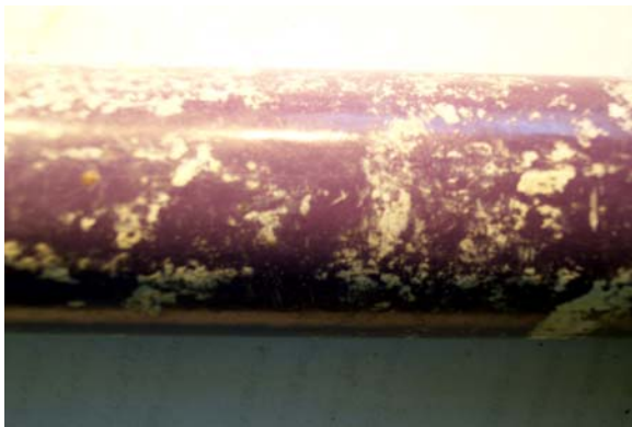
Figure 40. Epoxy-coated dowel (purple). (a) General view of the center region; (b) Corrosion was verified at the end region, underneath the epoxy seal.
