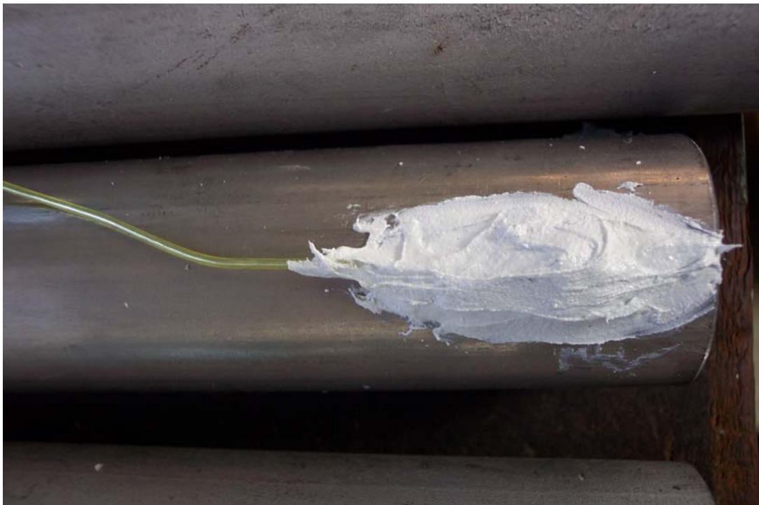
Figure 8. Electrical connections made to the stainless steel hollow specimens. Connections were made at the side of the dowel (a) and sealed with epoxy (b) before casting.
