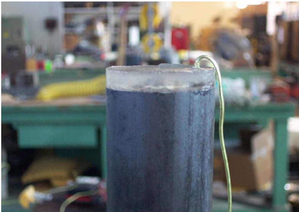
Figure 7. Electrical connections made to the dowels (a) before casting them in the concrete in order to perform half-cell potential and Linear Polarization Resistance experiments. Connections were sealed with epoxy (b) before casting.
