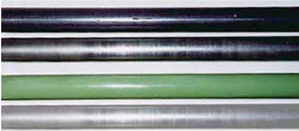
Figure 3. Steel dowel types investigated in Phase I. From top to bottom: carbon steel, stainless steel clad, carbon steel coated with bendable epoxy, and stainless steel hollow.
