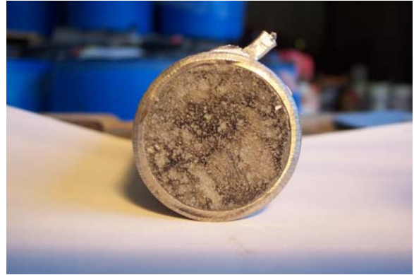
Figure 39. Stainless hollow dowels. (a) General view of the center region below joint; (b) End region showing grouted core.
