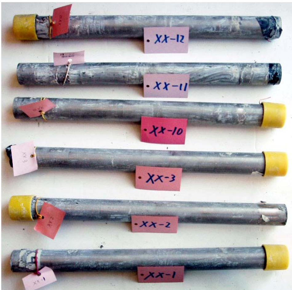
Figure 25. Appearance of stainless clad bars after tests.
