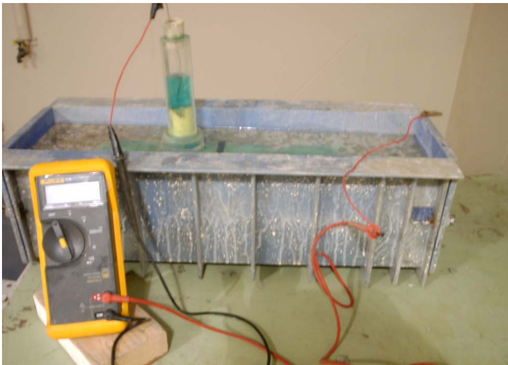
Figure 5. Half-cell potential test using a high impedance (10 Meg-Ohm) voltmeter, and a copper/copper sulfate reference cell.
