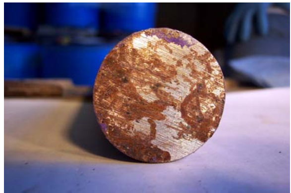
Figure 40. Epoxy-coated dowel (purple). (a) General view of the center region; (b) Corrosion was verified at the end region, underneath the epoxy seal.
