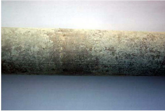
Figure 39. Stainless hollow dowels. (a) General view of the center region below joint; (b) End region showing grouted core.
