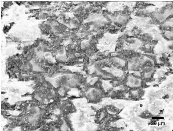
Figure 46. Hollow stainless steel samples: (a) view at the surface, 100×; (b) same region, 300×; (c) detail of the surface condition, 1000×. The surface appears rough, but no signs of corrosion damage were observed.
