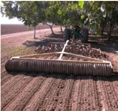
Figure 3. Spring tooth harrow breaking up the soil surface in an orchard. Photo: Terry L. Prichard
