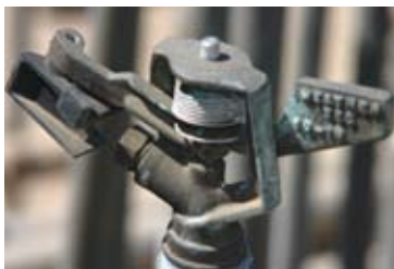
Figure 1. Close-up of an impact sprinkler head with the nozzle and orifice size (7/16) stamped on the nozzle. Photo: Lawrence J. Schwankl.
