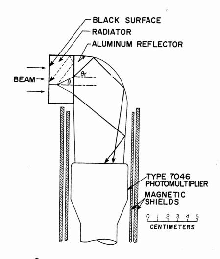
Fig. 2. Schematic diagram of Fitch-type broadband velocity-selecting counter.
