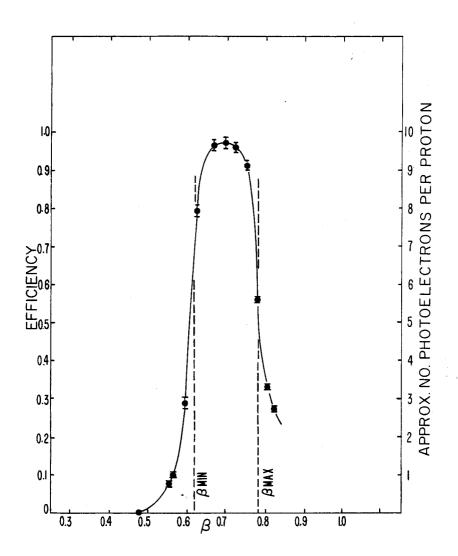
Fig. 3. Efficiency versus β for the Fitch-type counter illustrated in Fig. 2. The efficiencies were determined by placing the radiator between two scintillators of a counter telescope.
