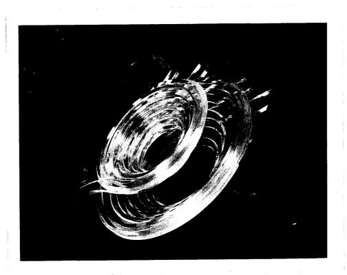
Fig. 1. Array of 16 scintillation counters for high-energy particle-scattering experiments.
