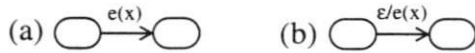
Figure 7. (a) A CSP event with input data, e?x , is modeled in UML State Machines as a state transition event with no action. (b) A CSP event, e , with output data, e!x , is modeled as a null state transition event that results in action e .
