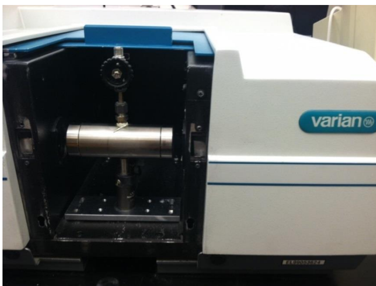
Figure 5.2 Side view of high pressure absorption cell with base in Cary 500 sample cavity.
