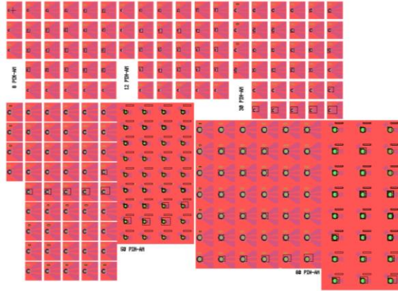
Fig. 11.12. Complete optical mask layout for photon-trapping MQWs PDs. Devices diameter ranges between 100 \mu\text{m} -8 \mu\text{m} with a variation of photon-trapping designs.
