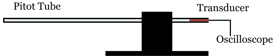
Figure 3.6: Simple schematic of a Pitot tube. The Pitot tube is inserted in the flow to collect a sample. The output from the pressure transducer is recorded by an oscilloscope. The entire assembly is mounted on to a 3D stage controlled by stepper motors to probe the entirety of the beam.
