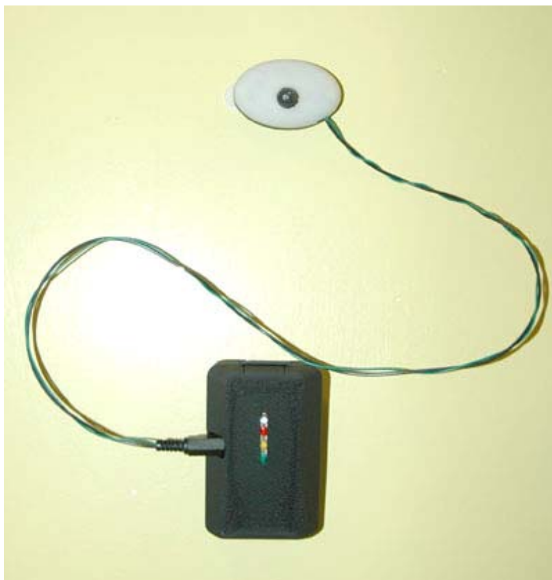
Figure 11: Price indicator mote with red, yellow, green and blue LEDs, and a motion sensor
