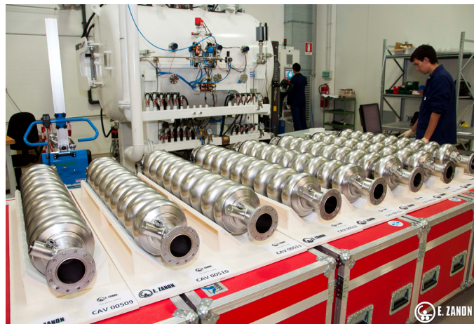
Figure 2.2: A set of pre-series XFEL cavities at the company E.Zanon.
