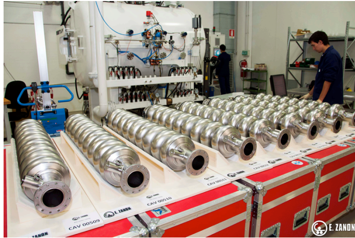
Figure 1.1: A set of pre-series XFEL cavities at the company E.Zanon.
