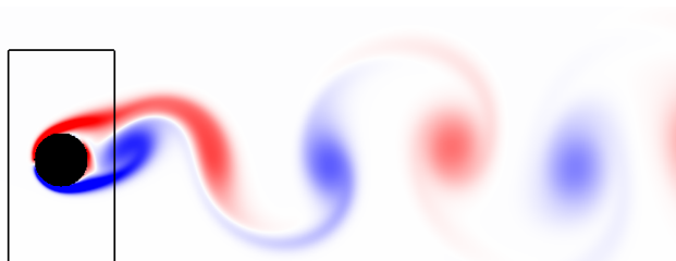
Figure 8: Vorticity generated by an oscillating cylinder in a cross-flow at tU_\infty / D = 100 for Re = 185 . The plotted vorticity is between -5 and 5 .
