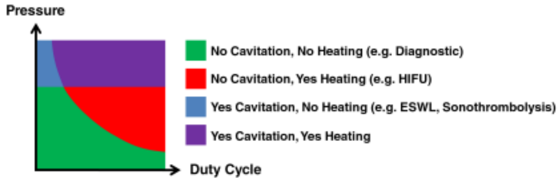
Figure 1.1 Four general ultrasound pulsing regimes. At a constant temperature and frequency, the production of cavitation or appreciable heat by ultrasound is a function of the acoustic pressure and duty cycle of the ultrasound. Achieving either heating, or cavitation, or both, or neither are all possible by tailoring the pulsing scheme. The independent parameters are frequency, pressure, pulse length (# cycles), and duty cycle (% time on).
