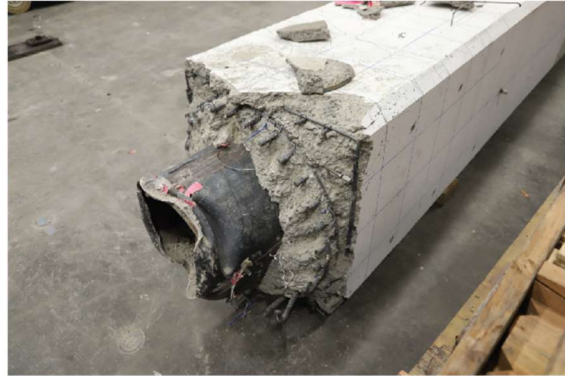
(h) Post-testing steel pipe damage.
