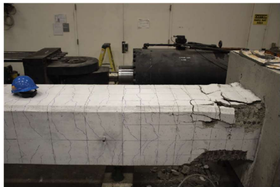
(l) Post-testing column-foundation joint (north side).
