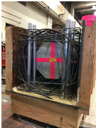
(c) Pipe cap at the column tip.
