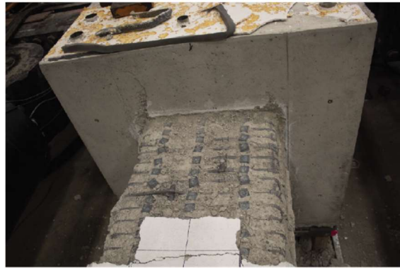
(p) Post-testing column-foundation joint (top face).
