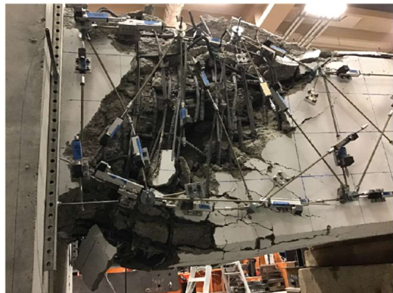
(j) Instrumentation failure post-testing.
