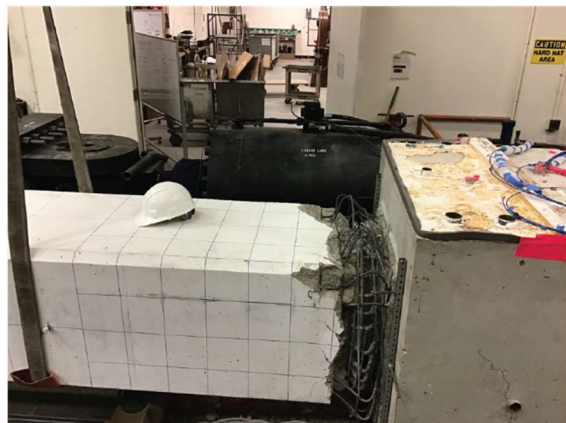
(f) Post-testing column-foundation joint (north side).
