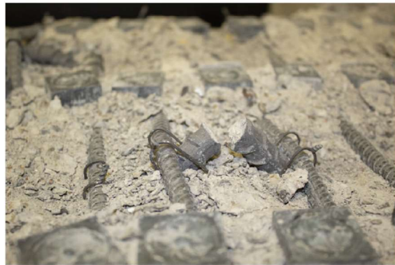
(p) Post-testing column-foundation joint (top face).
