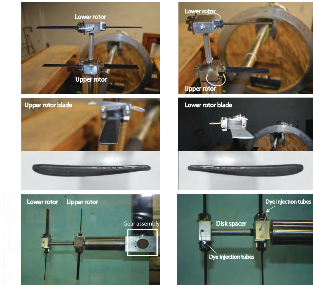
Figure 2.2: Coaxial rotor model assembly with axial rotor spacing of H/R = 0.8 : two-bladed (top-left) and one-bladed (top-right), upper rotor blade (middle-left), lower rotor blade (middle-right), location of gearbox (bottom-left), and closer view of disk spacer (spacer 7) and the dye injection tubes between the hubs and the blades (bottom-right).
