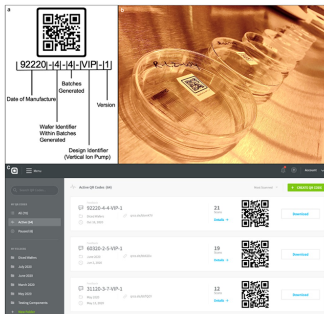
Fig 2. QR code tracking system. (a) A detailed breakdown of the unique identifier’s nomenclature that is tied to a QR Code, and (b) label device container with unique identifier and QR Code. (c) User interface subscription-based desktop application used to generate QR Code. Fig 2C provided through courtesy of QR Code Generator.
