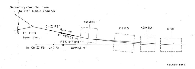
Fig. 6. Beam switching in the channel II second focus area for the 25-inch hydrogen bubble chamber.
