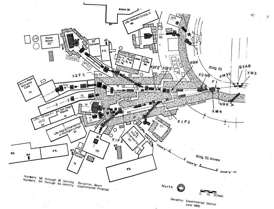
Fig. 3. Plan view of dual-channel external proton beam facility.
