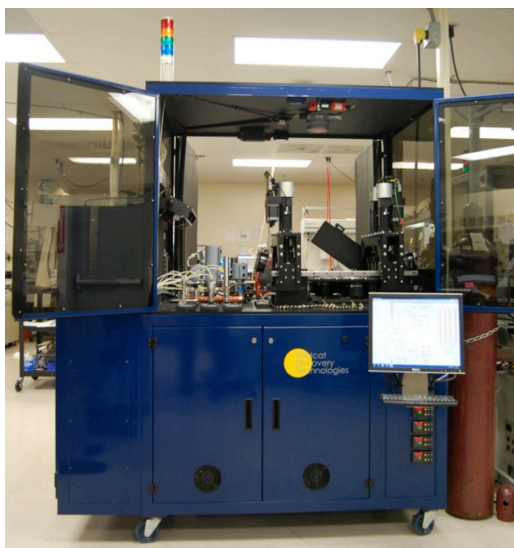
Figure 4.S13. High-throughput multicomponent adsorption instrument.
