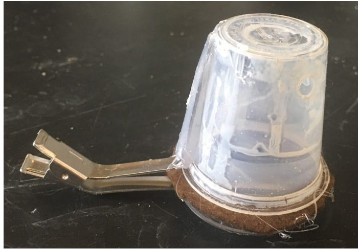
Figure 1: The fluon-coated clip cage used to contain the insects on the leaf and ensure the establishment of the footprints. It is composed of a hair clip (Walmart 6 pack of Goody Hair clips), the bottom of a small petri dish, and a small plastic cup with a 4 cm diameter at the top and 4 cm tall, then fluon coated on the inside to prevent insects from climbing. During preliminary experiments, we observed 90% of the lady beetles to be on the leaf using this method, with the remaining 10% on top of their compatriots rather than the leaf. Of these, 25% were observed in motion at two-minute intervals during the first hour.
