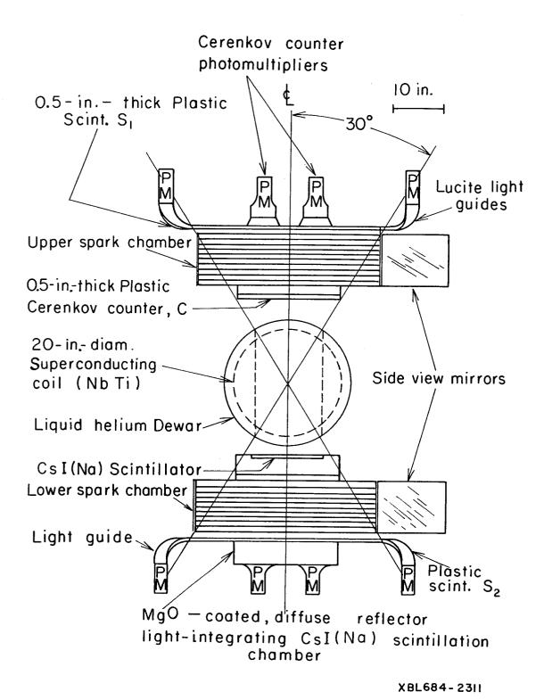
Fig. 1. Front view of charge-composition experiment.
