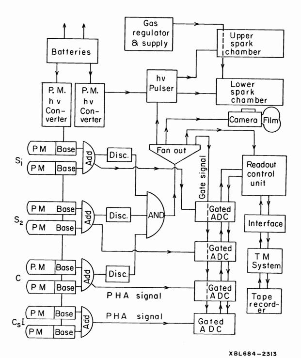
Fig. 3. Proposed electronics logic for charge-composition experiment.
