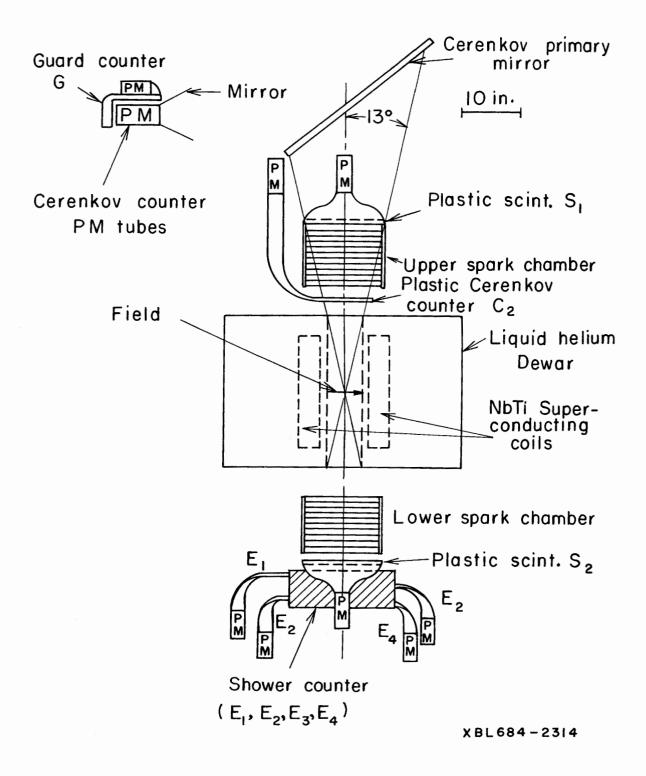
Fig. 4. Front view of electron experiment.
