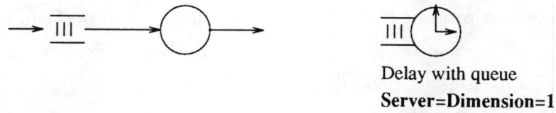
(a) single server queuing network and its Workbench specification
