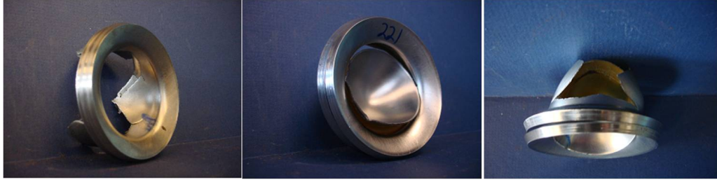
Figure 3.7: Samples after severe fracture: Experiment S02 (left): two plates without polyurea in between, Experiment P04 (middle): Sandwich structure front side, which received the impulsive load and did not fracture at the center, Experiment P04 (right): sandwich structure back side, severely fractured.
