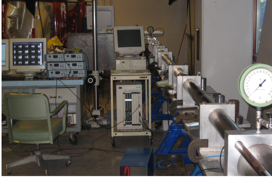
Figure 6.3: Experimental setup - 3" Split Hopkinson Pressure Bar in the high strain rate lab at UCSD's CEAM
