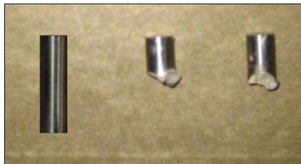
Figure 4.5: The projectile before and after the penetration. Eroded projectiles are from the experiments on bare ceramic samples.
