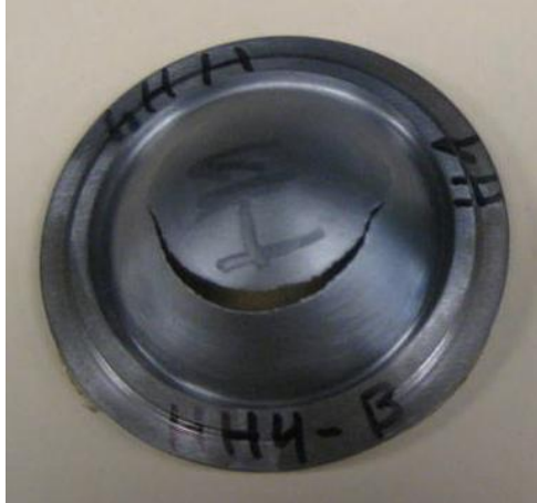
Figure 3.20: The back plate from the experiment HH4 after the impact test. The fracture does not occur at the center. This trend, which is predicted by the numerical model, is observed in a few, but not all, of the tested samples.
