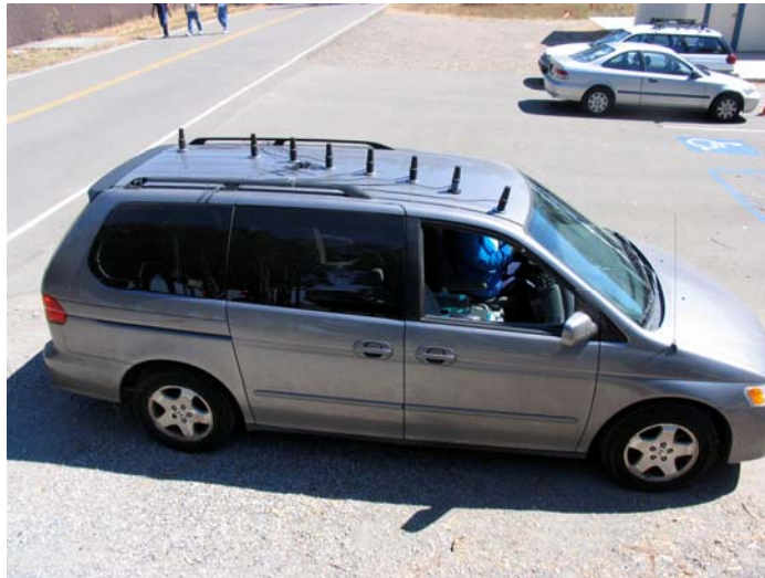
Figure 3.11 Antenna placements with 8 active OBUs on one vehicle
