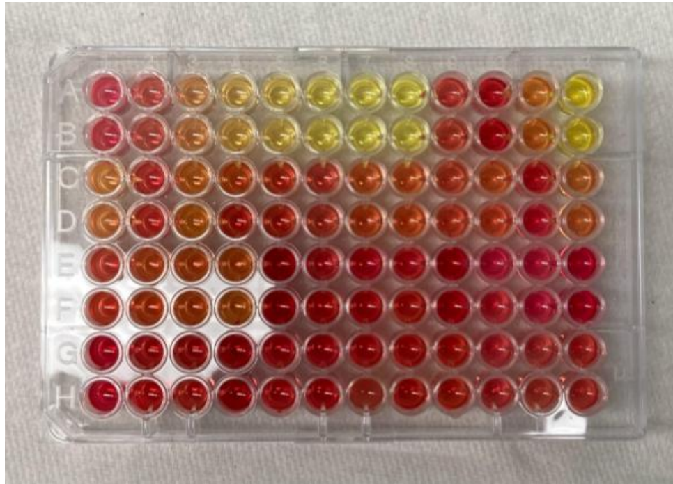
Figure 3.4. A 96-well plate after completion of the collagen assay protocol. This is inserted into the scanner for optical quantification of total collagen content, where a darker red in the well indicates higher collagen content.
