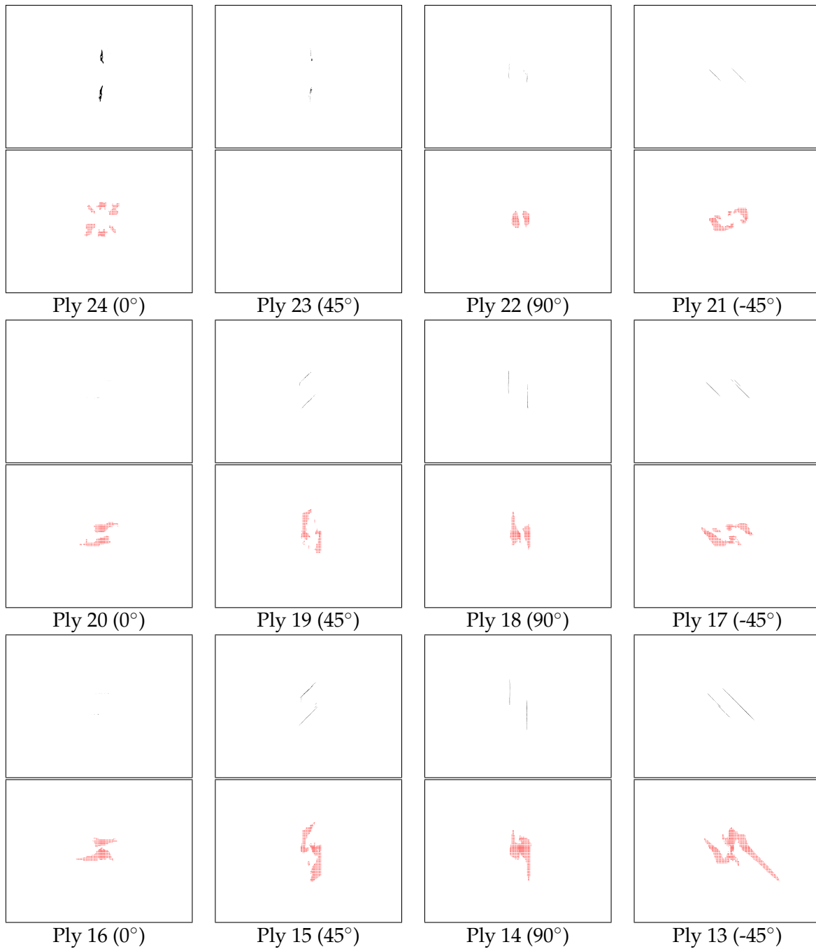
Figure 4.20: Impact on a 24-ply flat laminate. Correlation of (top) CT-scan results and (bottom) Matrix damage predicted by the IGA simulation for plies 13-24. Ply 24 is at the top of the laminate (impacted side). Each frame represents a 80 mm \times 60 mm area in the center of the panel.
