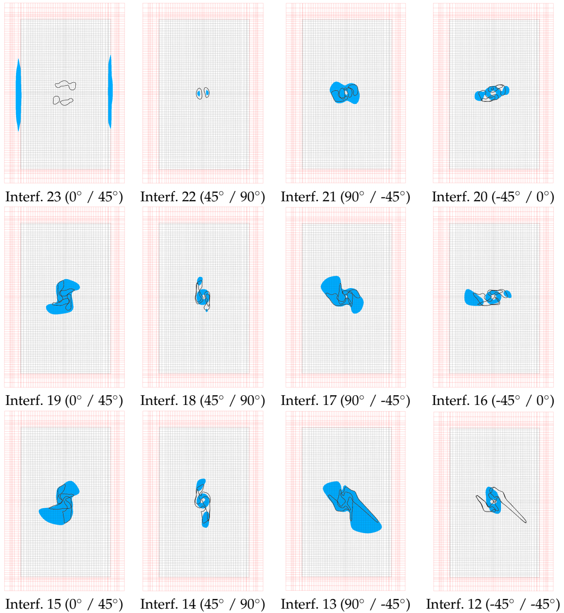
Figure 4.16: Impact on a 24-ply flat laminate. Correlation between matrix damage and delamination predicted by IGA simulation for cohesive interfaces 12-23. Cohesive interface 23 is at the top of the laminate (impacted side). The black solid line represents isocurves corresponding to d_2=0.5 , while the highlighted area represent the sub-domain of cohesive interface where d_{coh} \geq 0.5 .
