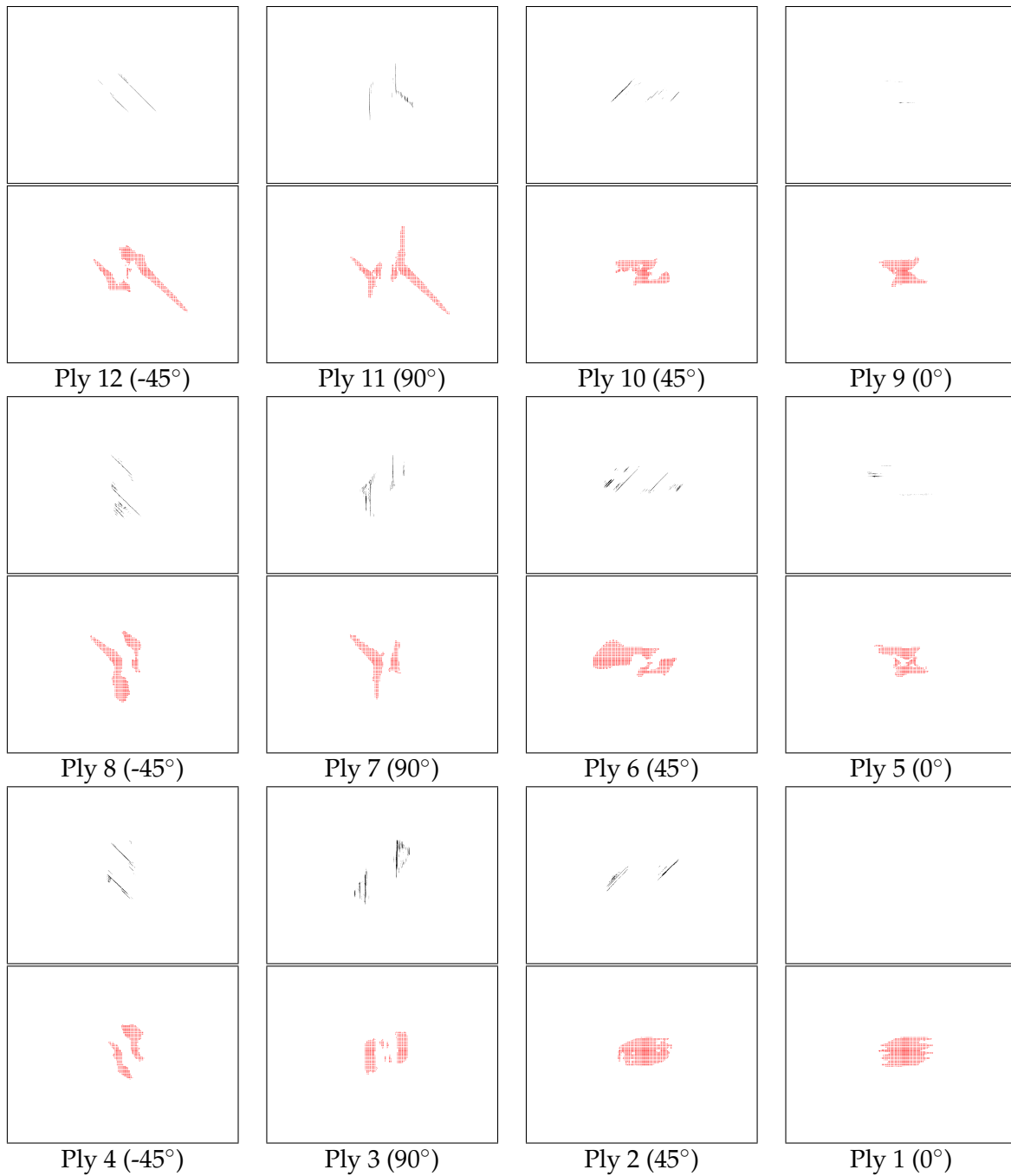
Figure 4.21: Impact on a 24-ply flat laminate. Correlation of (top) CT-scan results and (bottom) Matrix damage predicted by the IGA simulation for plies 1-12. Ply 1 is at the bottom of the laminate (non-impacted side). Each frame represents a 80 mm \times 60 mm area in the center of the panel.
