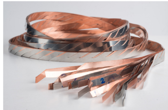
Fig. 25. Roebel cable. Source: Photo courtesy of CERN.
