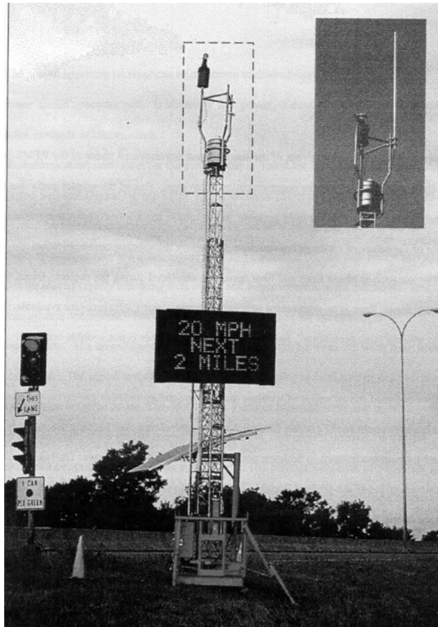
Figure 1-1. PTMS deployed on a skid
