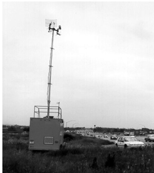
(b) Surveillance trailer alongside of I-5 freeway
