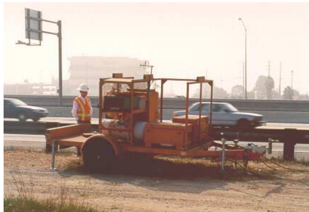
Figure 1-4. Ramp meter trailer at Grand Avenue alongside I-5 Freeway
