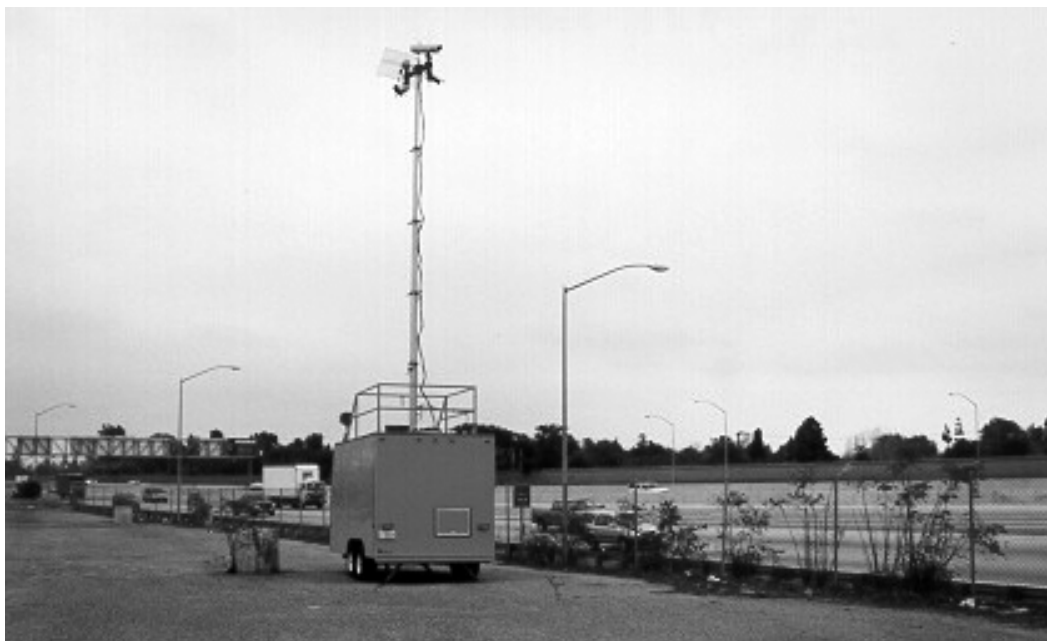
Figure 4-4. Surveillance trailer at Main Place looking south along I-5
