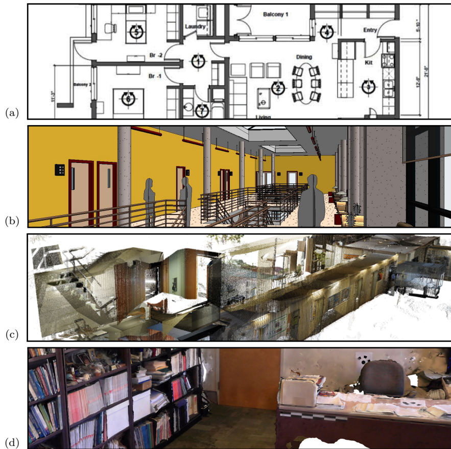
Figure 11. Examples of present forms of indoor representation: (a) CAD, (b) BIM, (c) point cloud, and (d) textured mesh. Image credits: (a) public domain, (b) Autodesk, and (c) and (d) Jorge Chen, CC BY-SA 3.0.
