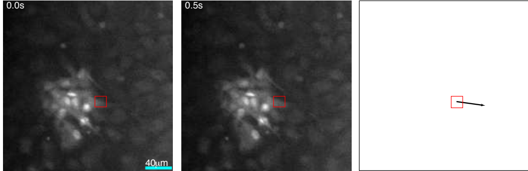
Figure 2.2: The optical flow algorithm. A window \Omega in the same location in two subsequent image frames is used to compute a displacement or flow vector (arrow) for the pixel at the center of the window. Only image intensity values in \Omega are used for the calculation. Vectors are computed for each pixel in an image frame except in border regions where \Omega falls outside of the image. Given the position of the pixel as (x, y) at t seconds, (x, y, t) , the displacement vector defines the motion of the pixel at the subsequent frame at \delta t seconds as (x + \delta x, y + \delta y, t + \delta t) .
