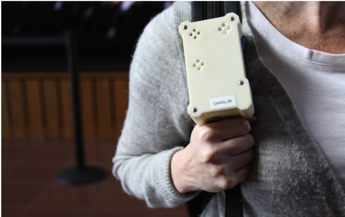
Figure 4.6. These prototype boards could be carried attached to a backpack strap, secured to a bicycle frame, or carried in hand.
