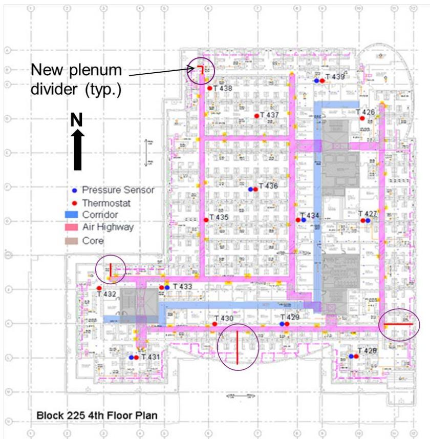
Figure 4-16. Plan view showing installation of plenum dividers at four locations
