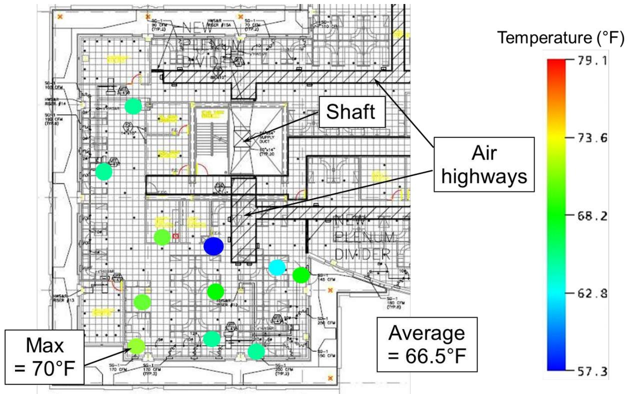
Figure 4-17. Diffuser discharge air temperatures: B-225, southwest zone, 4<sup>th</sup> floor, 9/20/2013
