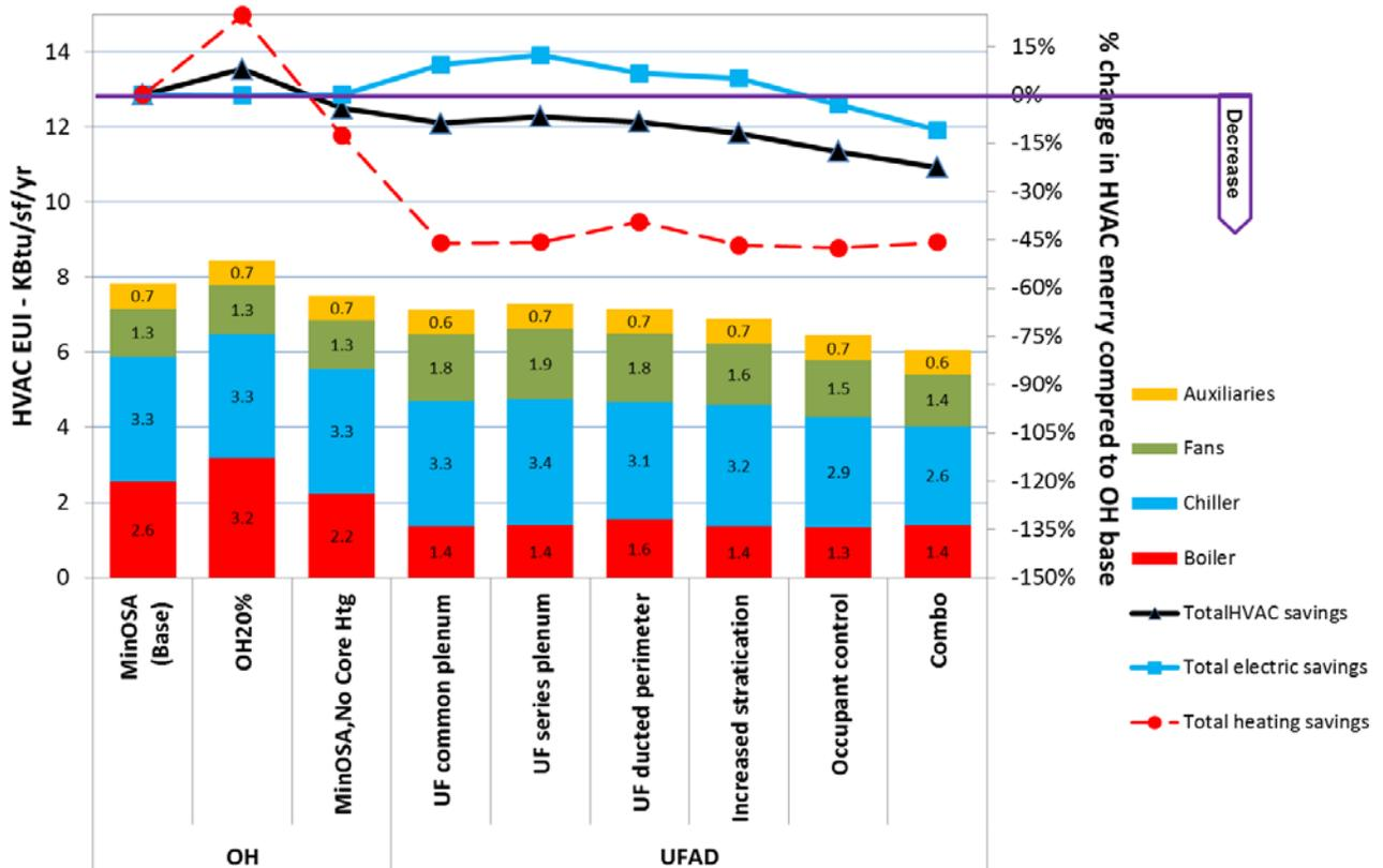
Figure 5-4. Results of UFAD vs OH simulation study [Webster et al. 2012]
