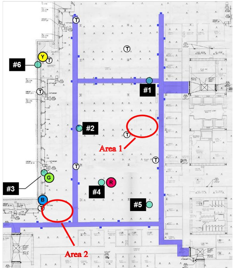
Figure 4-5. Hobo plenum and stratification logger locations
