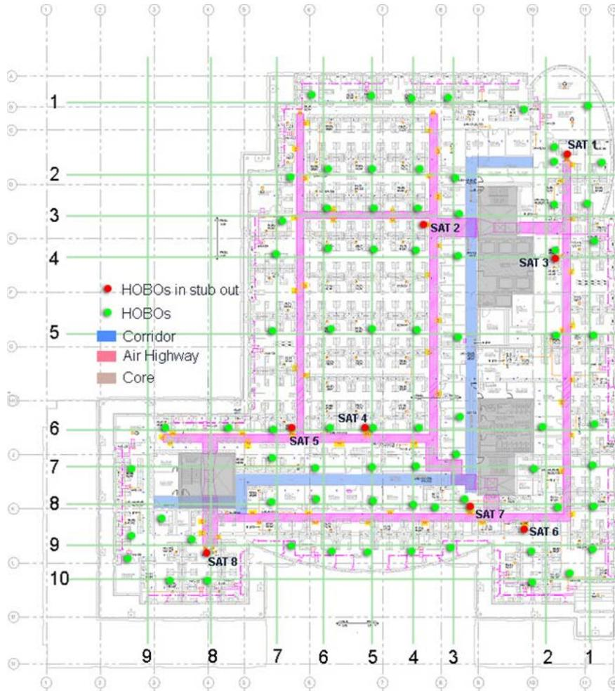
Figure 4-10. Plenum temperature measurement locations: Block 225, 4<sup>th</sup> floor
