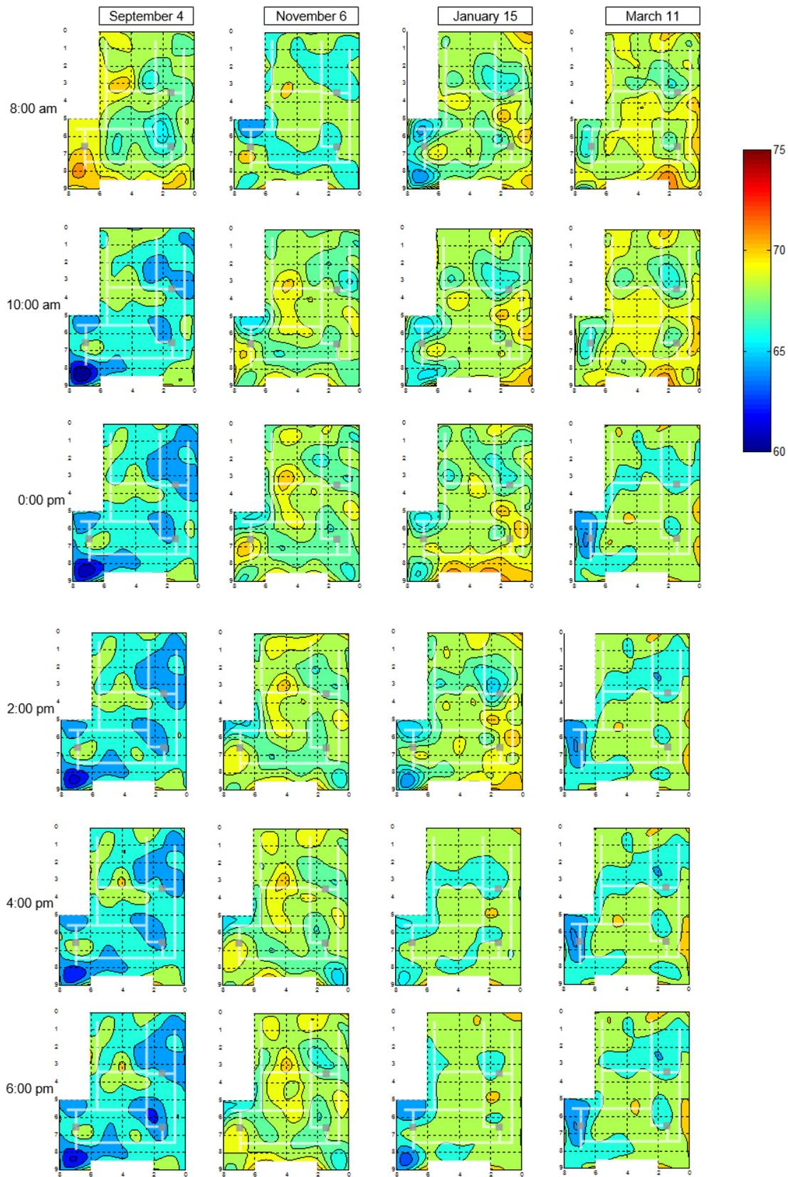
Figure 4-11. Plenum Temperature Contour Maps every 2 hour from 8:00am to 6:00pm
