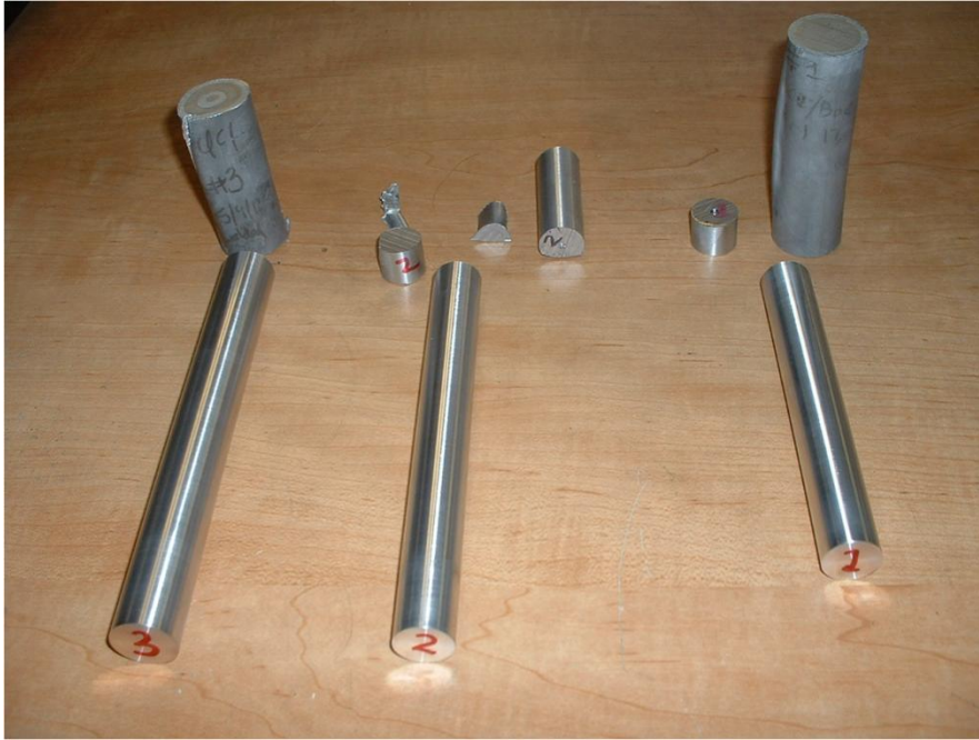
Figure 3 Billets Consolidated from Cryomilled Powders. The portions at the top left and right of the image are still in the HIP canister. Other sections have had the can removed by lathing.
