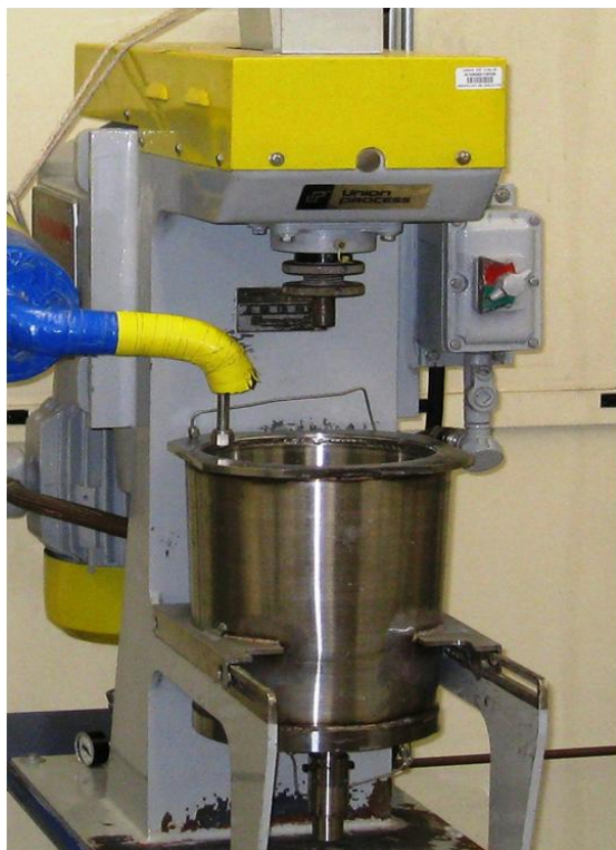
Figure 1 Cryomilling Apparatus. Shown are the body and motor casing, liquid nitrogen connection, and milling container with bottom valve attached. Not shown is the attrition arm or lid.
