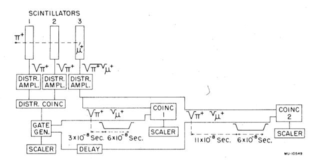
Fig. 4. Block diagram of the electronics.
