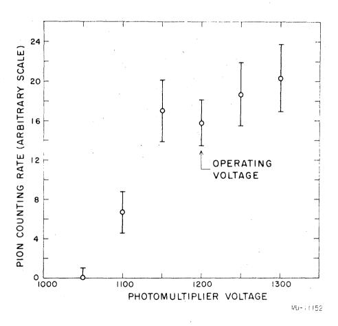
Fig. 8. Voltage plateau for photomultiplier on third scintillator.
