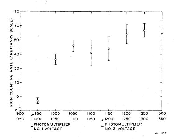
Fig. 9. Voltage plateau for photomultipliers on first two scintillators.
