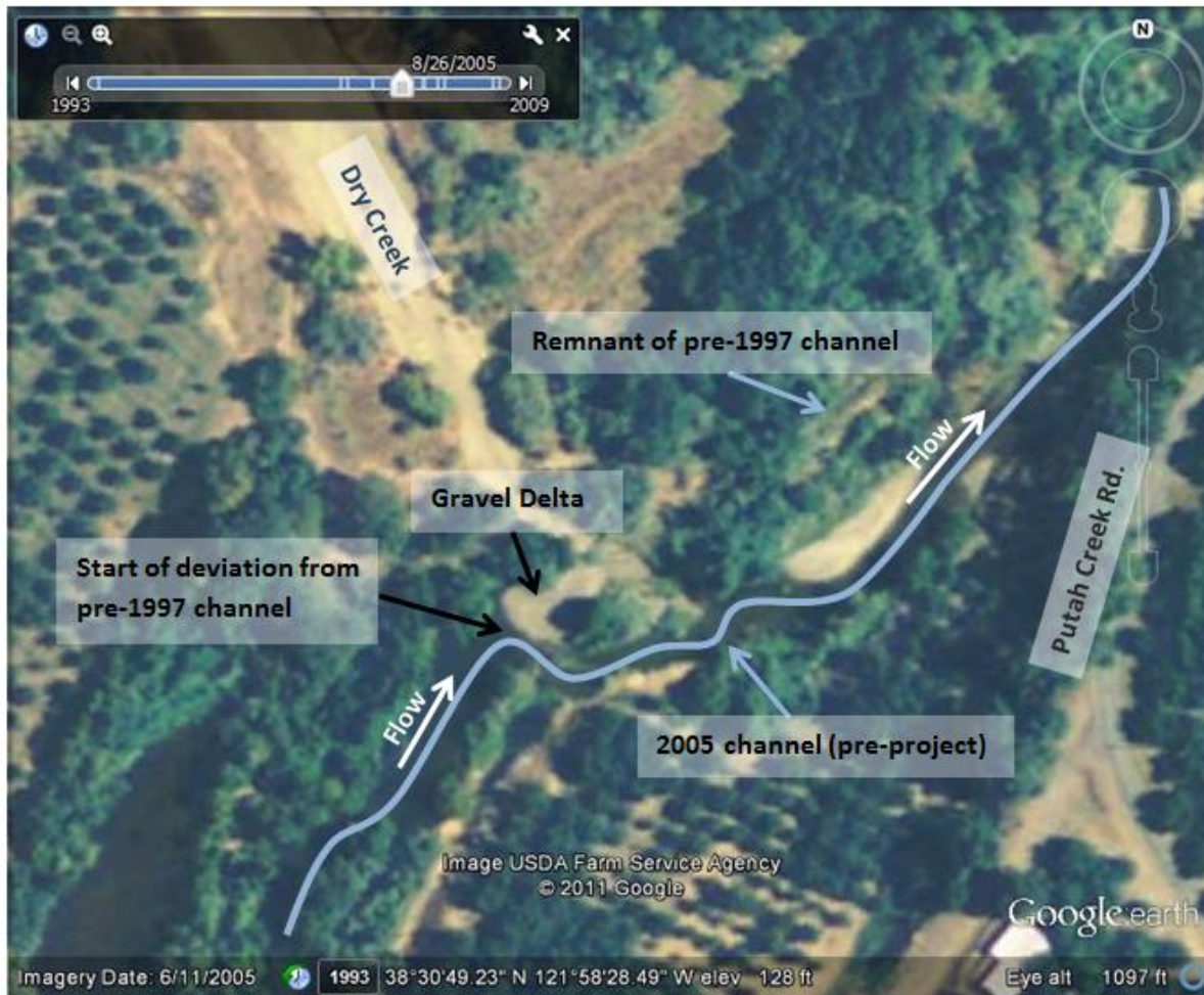
Figure 1. This 2005 Google Earth photo shows the gravel delta formed at the confluence of the creeks.
