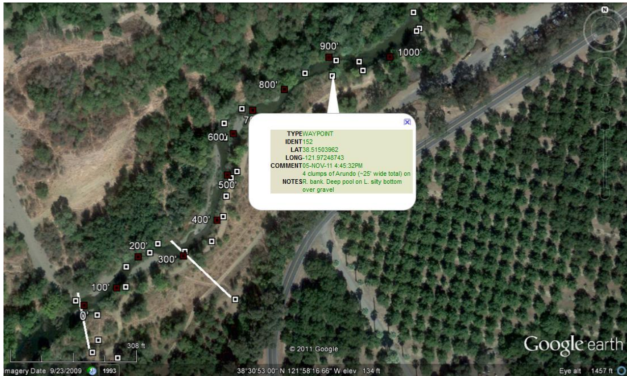
Figure 7. Screenshot of Google Earth showing our waypoints as squares. Red squares are the dividers of the 100 foot sections. White lines are the two transects we surveyed in 2011.
