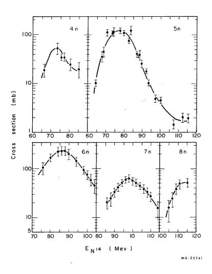
Fig. 2. Excitation functions for  $N^{14}$ , xn reactions on  $Pt^{198}$ .
