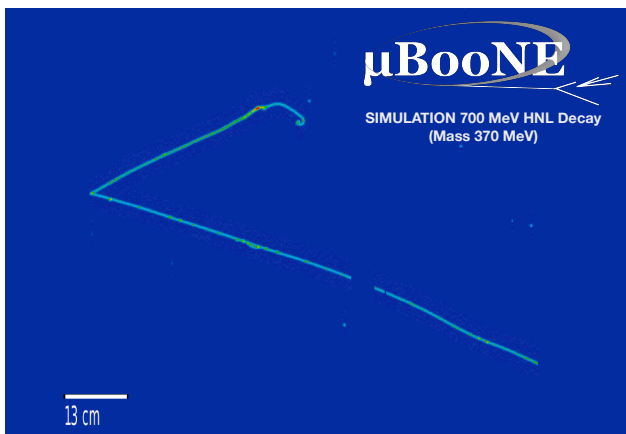
FIG. 2. Display of a \mu\pi decay for an HNL with a mass of 370 MeV, showing the signals measured at the collection plane. The horizontal axis represents the wire-number, and the vertical axis represents time. Colors show the charge deposition measured on the wires. The gap in the longer track is due to a set of unresponsive wires.
