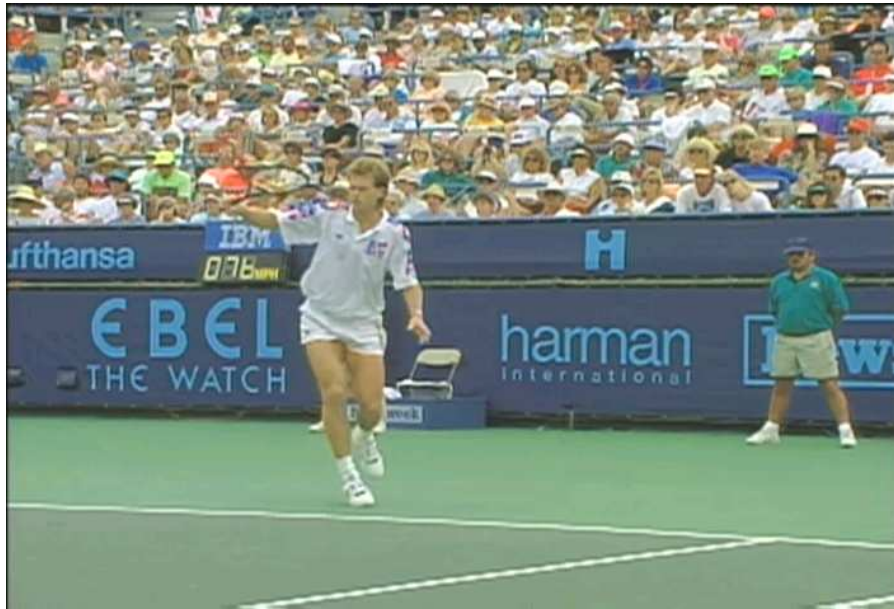
(a) Lost frame number 35 of Stefan. Whole frame concealment by JM decoder with frame copy.
