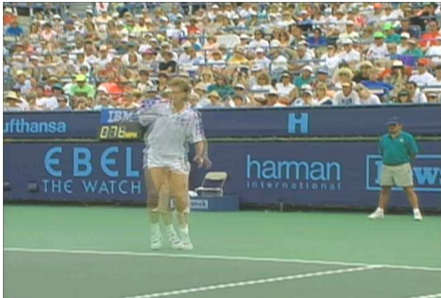
(b) Lost frame number 35 of Stefan. Whole frame concealment by FFMPEG decoder with temporal frame interpolation.
