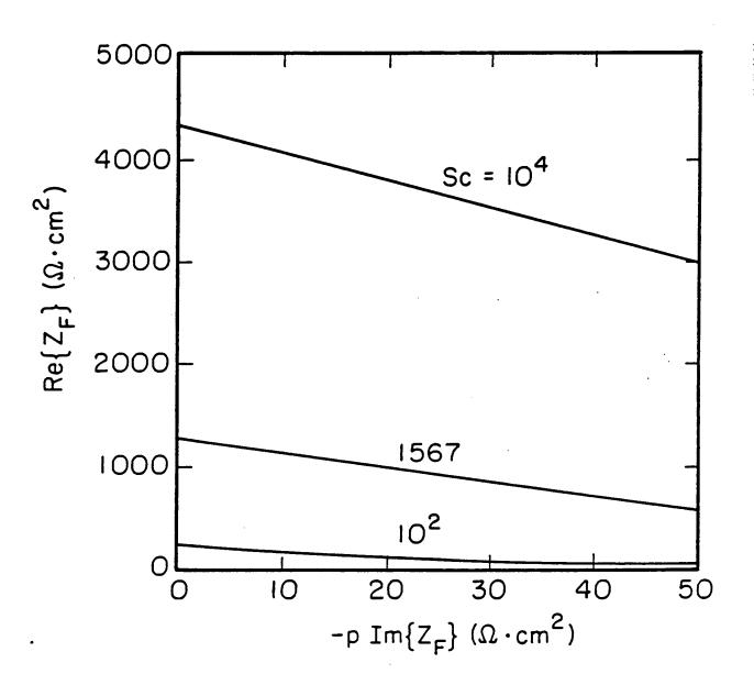
Figure 4. Smyrl plot of the low-frequency region of the faradaic impedance.
