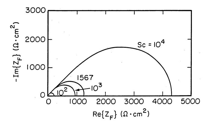
Figure 2. Nyquist plot of faradaic impedance as a function of Sc.
