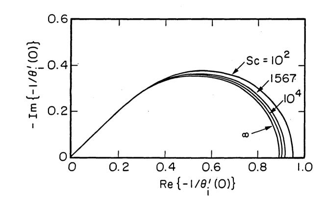
Figure 5. Nyquist plot of the dimensionless convective-diffusion impedance.
