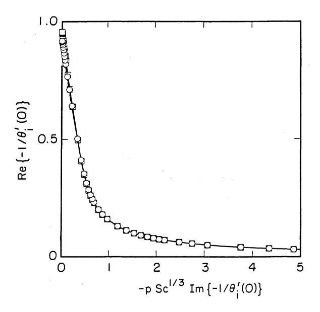
Figure 7. Plot of the dimensionless convective-diffusion impedance as a function of Sc covering a larger frequency range than figure 6 and with the abscissa stretched with the value of the Schmidt number.
