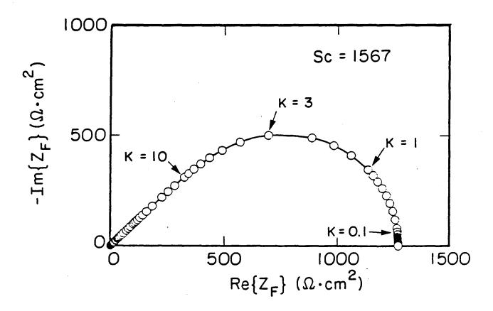
Figure 1. Nyquist plot of the faradaic impedance for the anodic dissolution of copper.
