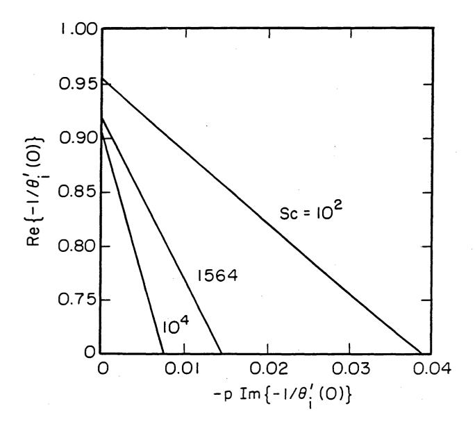
Figure 6. Smyrl plot of the dimensionless, convective-diffusion impedance for several values of Sc.
