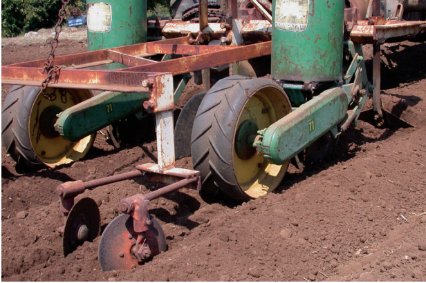
FIGURE 3. Soil cappers run behind the pack wheel create a loose “cap” of soil over the seed line. Photo: Jim Leap
