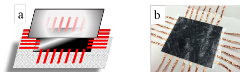
Fig. 1. (a) The nanocomposite is integrated with fabric using iron-on adhesives. (b) A picture of an actual fabric-based sensor is shown.
